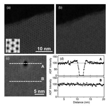
FIG. 5. High-resolution ADF-STEM image of MCM-22 zeolite recorded using 60 keV aberration-corrected STEM before the damage. The inset at the bottom corner is a portion of the same image after statistical improvement. (b) The sample in (a) after 35 s of beam exposure with 40 pA beam current. (c) ADF image of another area after hole formation under an intensive point beam. (d) Two line scans from the image in (c).
