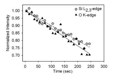
FIG. 4. Measured integrated intensity of the Si  $L_{2,3}$  and O K edge EELS spectra as a function of beam exposure time. Starting from edge onset, a 20 eV energy range was used for integration and the results were normalized to the initial spectrum. A 200 keV electron beam was used here.
