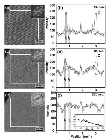
FIG. 2. (a) High-resolution TEM image of MCM-22 zeolite recorded after 25 s of 200 keV electron beam exposure. The inset at the top-right corner is FFT obtained from the highlighted area in the image. (b) Two line scans from the FFT shown in (a) labeled "A" and "C." (c),(d) Same area of the sample after 85 s of beam exposure. (e),(f) The area after 220 s of beam exposure. The inset in (f) is an evaluation of the ratio  $R = (I_c - I_a)/I_a$  as a function of exposure time with linear fit.
