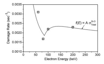
FIG. 3. Caparison of the measured degradation rate in MCM-22 zeolite with calculated total cross section,  $\sigma_{\text{Total}}^{\text{Si-O}}(E)$ , that includes both radiolysis and knock-on damage mechanisms.
