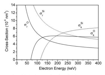
FIG. 1. Calculated crosssections for radiolytic movement and knock-on surface sputtering for silicon and oxygen atoms in the MCM-22 zeolite as a function of incident electron energy.
