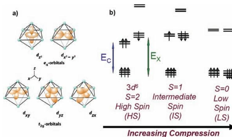
Fig. 1. (a) *3d* orbital alignments and their classification in octahedral field. *E<sub>c</sub>* is the crystal field splitting and *E<sub>x</sub>* is the Hund's rule energy. (b) Energy levels and occupancies for  $3d^6$  ions, such as ferrous iron. Ferric iron has configuration  $3d^5$  and the electron in the highest energy level is absent. Its total spin in HS, IS, and LS states are 5/2, 3/2, and 1/2 respectively.
